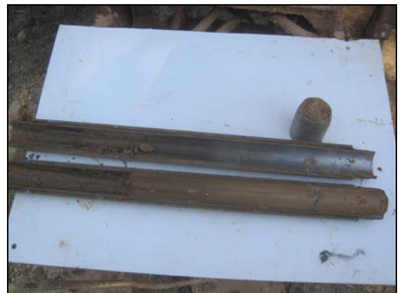
Foto 16: Sondeig S-3. SPT a 6,0 metres.
