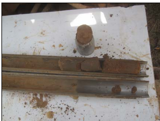
Foto 11: Sondeig S-2. SPT a 2,0 metres.
