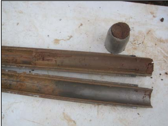
Foto 13: Sondeig S-2. SPT a 8,0 metres.
